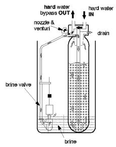
4 BACKWASH: During backwash, water flows UP through the resin tank (FIG. 8) at a fast rate to flush iron minerals, dirt and sediments from the bed and to the drain. The bed lifts and expands for good cleaning.
